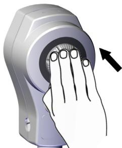
If the time delay is fitted, the unit cannot operate a full dose again until the green indicator in the middle of the pusher has fully returned.
