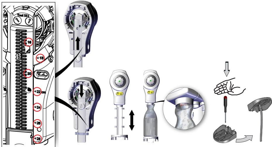
For the spray bottle version set correct height of the bottle base. Ensure the spout is inside the neck of the bottle.
