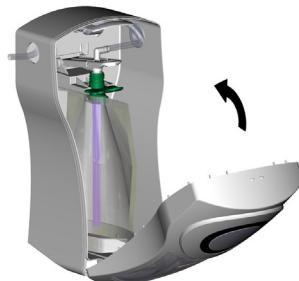
Pop up the pouch lever in the cabinet. Hold the 1.5ltr pouch by its neck and insert it into the pouch chassis. Pull the lever back down and click it firmly to secure the pouch.
